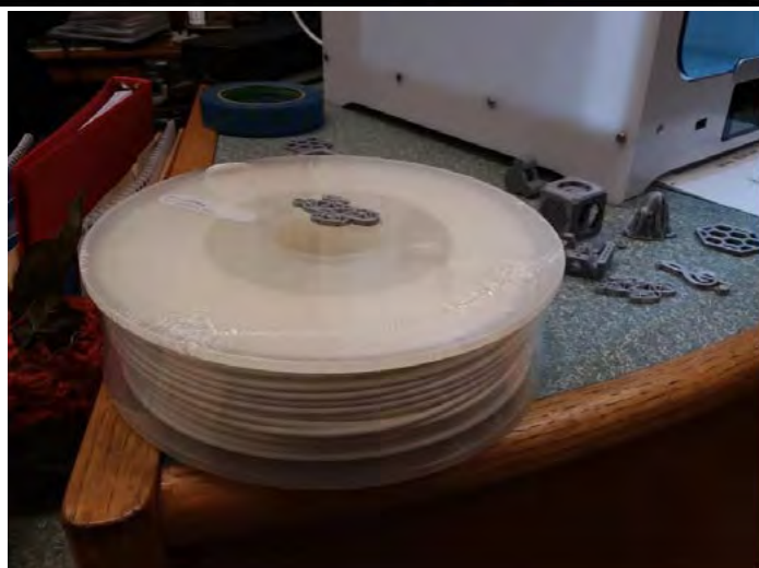
A spool of gray plastic rod used as the "ink" to the 3D printer.
