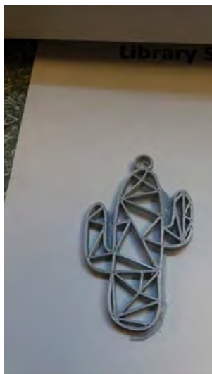
3D printer lays down bed of plastic to anchor the cactus as it builds its layers.
